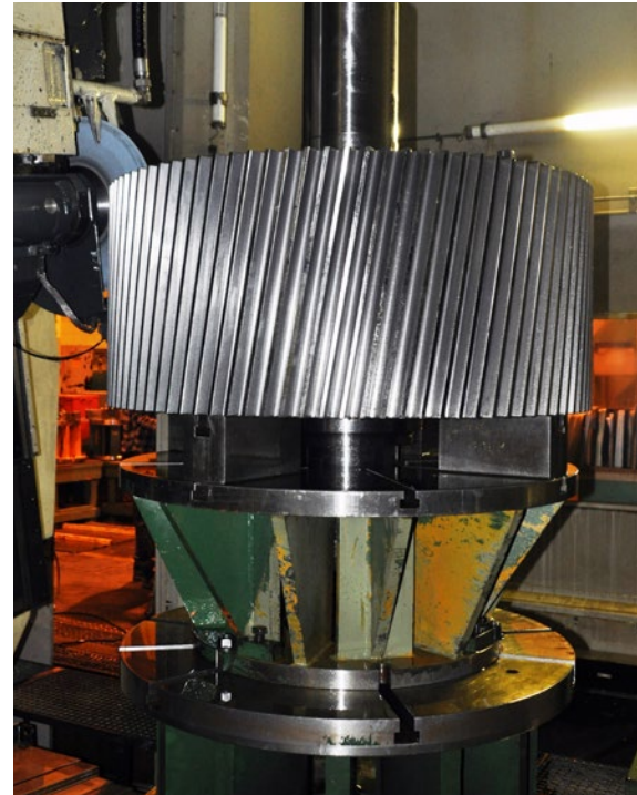
MR re-cut low speed gear at finish grind.
